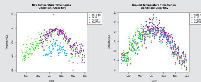
**Figure 4:** (Left) Infrared sky temperature time series. (Right) Infrared ground temperature time series.
