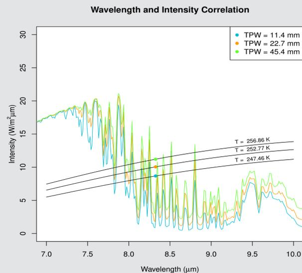
**Figure 1:** Based on calculations using MODTRAN [2]. Blue, orange, and green curves relate to TPW of 11.4 mm, 22.7 mm, and 45.4 mm, respectively. Corresponding circles represent mean radiance of the spectral band between 7-10  $\mu\text{m}$ . Solid black curves show corresponding black body emission curves at the indicated temperatures.
