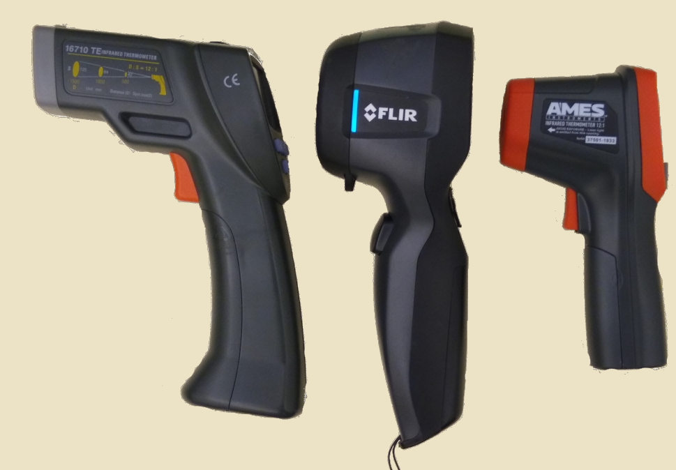
Figure 1: (Left) The three infrared thermometers used to collect data: (from left to right) 1610 TE, FLIR i3, and the AMES 12:1 Infrared Thermometer.
